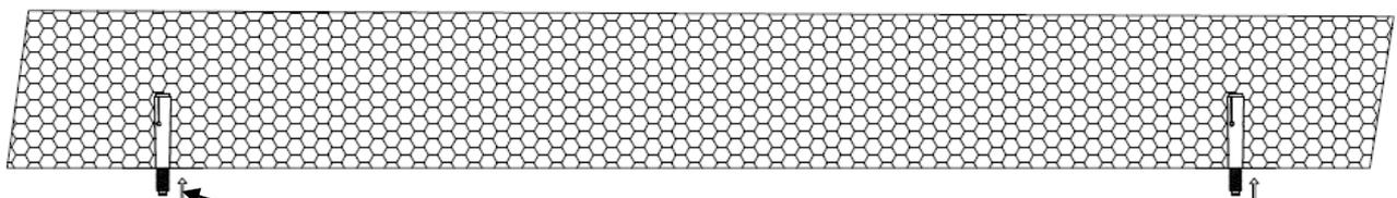
Fix the expansion screws in the wall
