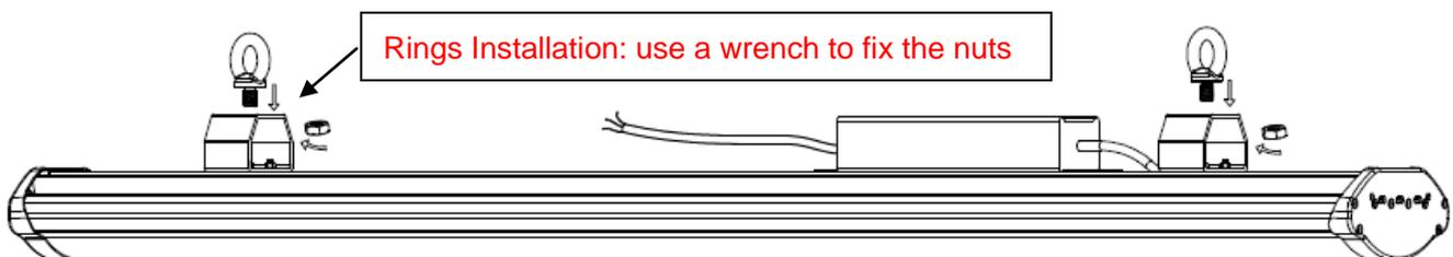
Adjust the interval space between the fittings according to actual
