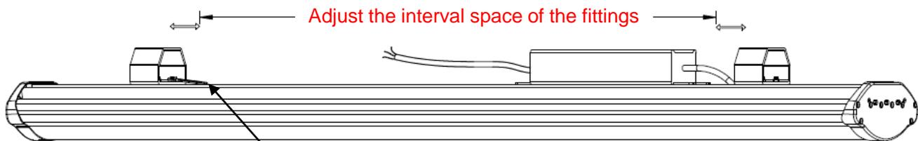
use a wrench to loosen the nuts, adjust their interval space and lock them
